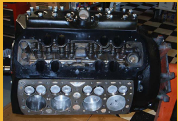
Pistons and valves tops coated. Springs coated to increase life against flexing
