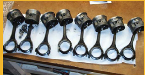
Pistons coated with thermal barrier, dry film lubricant and thermal dispersant
